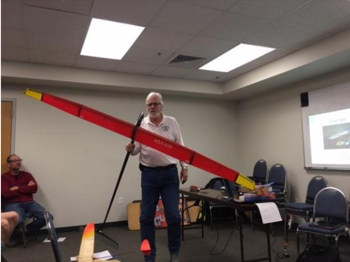
The wing tips of this model fold during the dynamic launch phase to minimize drag and then unfold to catch the thermals. Even with the multiple hinges the C-F torque tube wing spar construction essentially eliminates wing tip twisting in flight.
