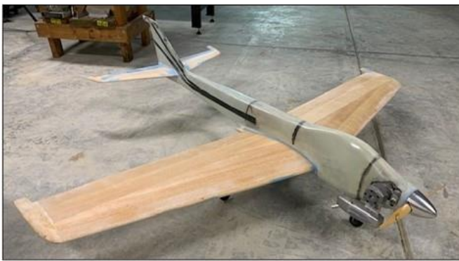
Carbon fiber reinforcements are visible in the laminate and the plane's clean lines are evident here
